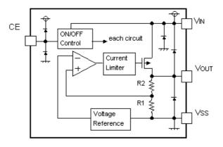
Fig.1: A phase compensation feedback system provides a very stable output, allowing low ESR capacitors to be used.
