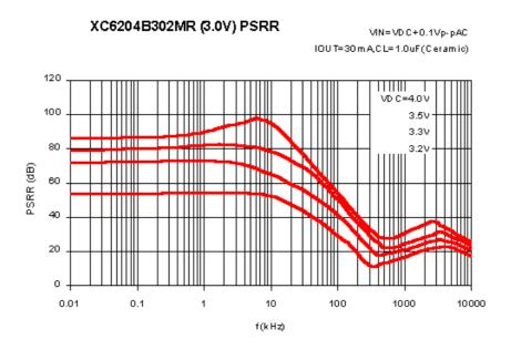
Fig.4: Ripple rejection (PSRR) is very important in high sped LDO regulators.
