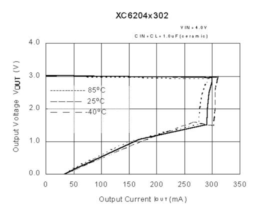
Fig.3: Small changes in temperature characteristic result in stable current control of typically 300 mA.
