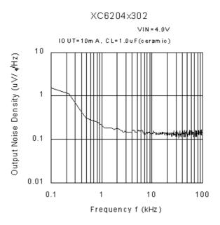
Fig.2: Output noise density.
