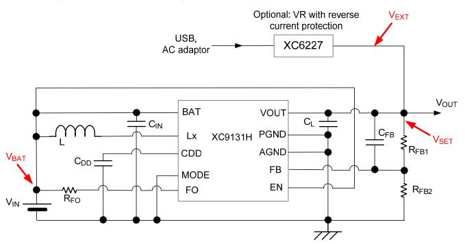
On the circuit diagram above, you can see that EN = 'High' (the IC is enable) and MODE = 'Low' (the IC operates in PWM/PFM mode). As mentioned previously, these voltage levels won't have to be adjusted while the circuit is operating.
